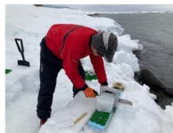
Making of Sea Ice Sample for the Strength Test in Utoro
